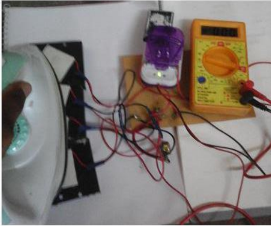
Fig 2: (a) charging the sample mobile battery using TEG by waste heat
