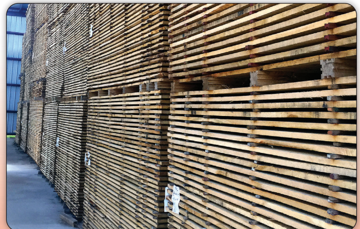
An example of proper sticker placement for stacking lumber.
