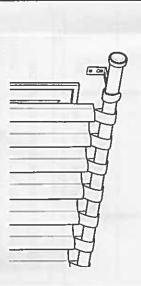
Lock rod in position by tightening screws into back of bracket.
