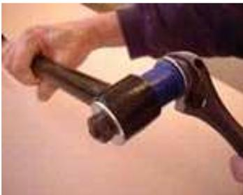
If you're really struggling - a long bolt, nut and two large washers can be used to wind the bush into place.
