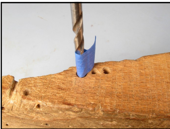
Drilled hole depth is determined by the location of the tape.
