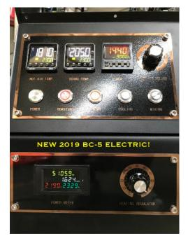
NEW FOR 2019: POWER METER: SHOWS THE WATTAGE, VOLTAGE AND AMPS BEING USED AT ANY GIVEN TIME. (PANEL LIGHTS UP WHEN TURNING THE HEATING REGULATOR UP)
