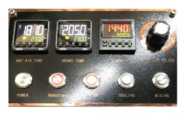
TWO OMRON TEMPERATURE CONTROLS FOR BT & ET ONE TIMER FOR TIMING ROASTS (RESET BUTTON ON LEFT BOTTOM)
