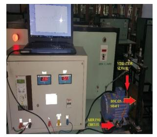
Figure 1. Test bench details; (right on motor) positions of the accelerometer, (right) load unbalance introduced on the disc mounted on the motor.
