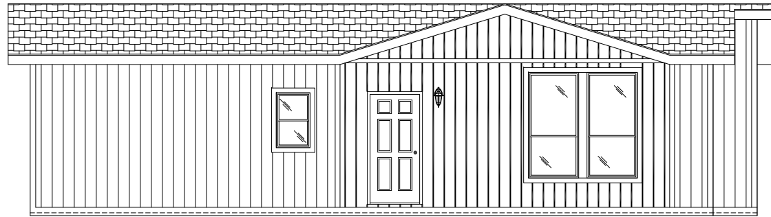
FRONT SIDEWALL W/NOMINAL 20'-0" DORMER
