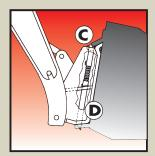
**Exclusive Bob-Tach system** Left to right, Bob-Tach frame **(A)** moves into attachment flange. **(B)** Handle **(C)** pushes down easily, pressing wedge **(D)** through frame and attachment hole for a solid connection.
