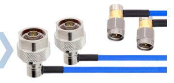
ConductRF PFT series of Low Loss, Performance flexible RF cable assemblies utilize a new dielectric material that eliminates what is commonly called the PTFE Knee that is the cause of Phase to vary with temperature in a non-linear fashion. The dielectric used in these cables provides for a more linear change in Phase as temperature changes, so the change variance is less impactful.
