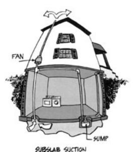
**Active Subslab** suction (also called subslab depressurization) is the most common and usually the most reliable radon reduction method. One or more suction pipes are inserted through the floor slab into the crushed rock or soil underneath. They also may be
