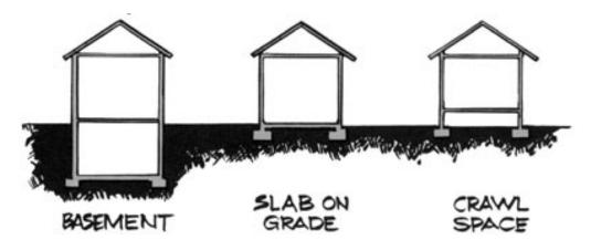
Radon reduction systems can be grouped by house foundation design. Find your type of foundation design above and read about which radon reduction systems may be best for your house.
