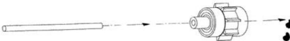
Place the chuck into the turbine and tighten by turning the chuck tool counter-clockwise.
