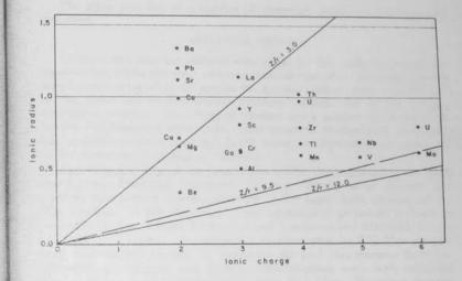
Figure I. Grouping of certain elements according to ionic potential
