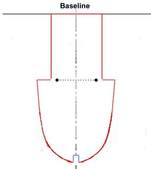
Figure 13. Making a horizontal cut to remove the extension.
