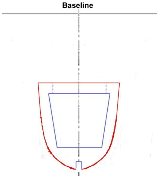
Figure 11. Cutting lines added to top part of rib.
