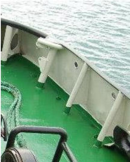
**Figure 22. Bulwark supports on a real tug, made from pipe and plate.**
