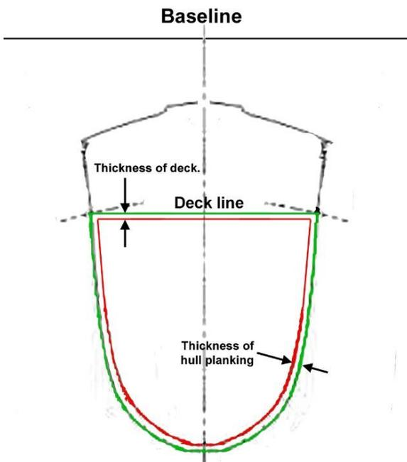
Figure 8. The rib outline modified for deck and planking thickness. The outer line is the original outline from the Body Plan; the inner line shows the shape required inside the hull.
