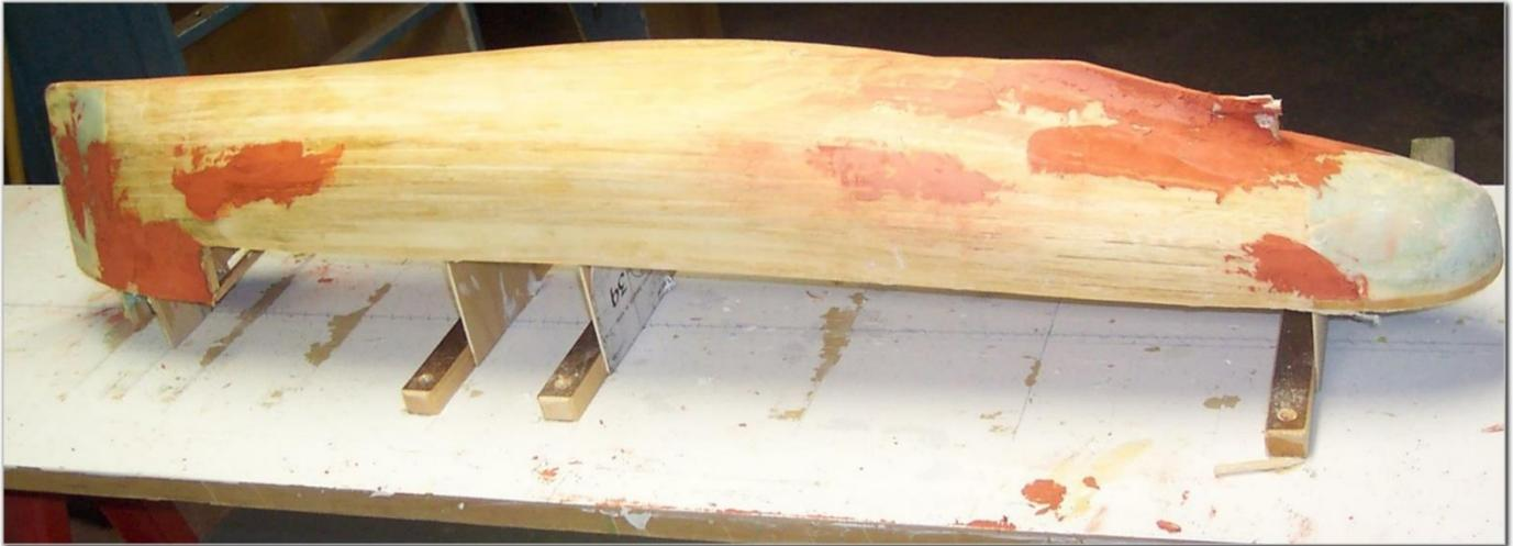
**Figure 21. Radley's (Steve M's dad) trawler hull after shaping of the bow and stern, removal of some of the rib extensions, and with Bondo applied. Ready for painting.**
