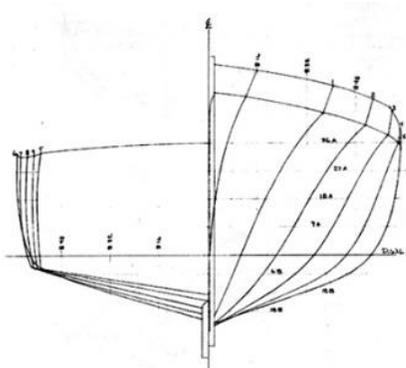
**Figure 19. A section through a hull of mixed type.**
