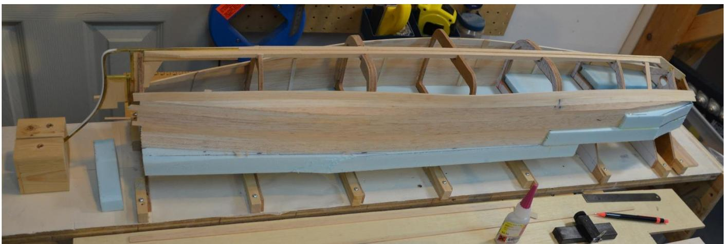
Figure 18. Roy's *Wahine* hull during planking. On this hull, blue foam insulation was used along the top edge of the hull, and planking started from there.
