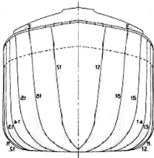
Figure 5. Full-width template of the bow portion.
