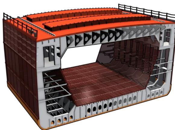
Figure 2. Section through a ship's hull.
