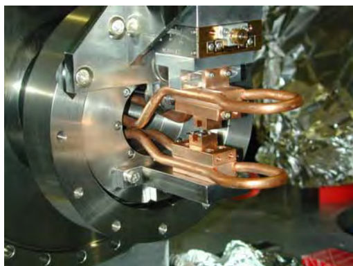
FIGURE 3. Shows water cooling tubes and crystal mounts.
