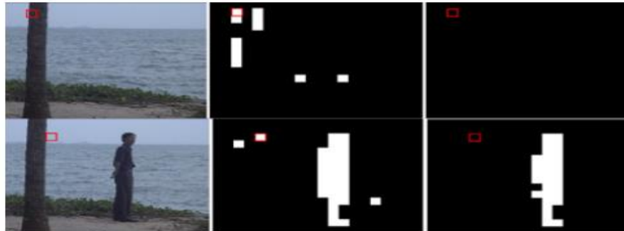
Fig. 1: Block-based background subtraction results with WATERSURFACE . Column 1: Original images. Column 2: Block-based results of HCB. Column 3: Block-based results. [10]
