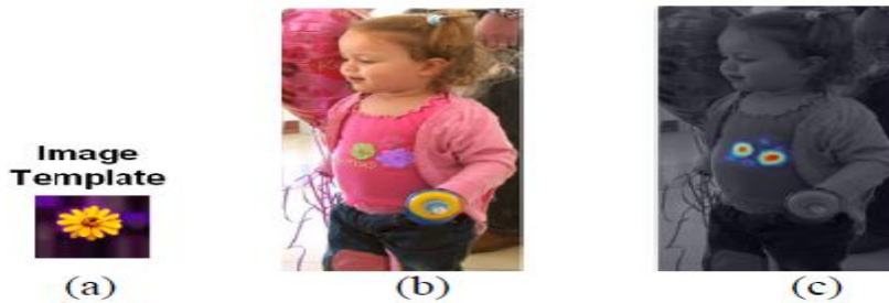
Fig. 3: (a) Image template (b) Image against which it is compared (c) Detected object superimposed on gray-scale image
