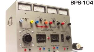
The **Model BPS-104** consists of various AC and DC power supplies rated for use with Hampden Series 100 fractional horsepower machines as well as general laboratory use. The **Model BPS-104** consists of one AC ammeter, one AC voltmeter, one DC ammeter, and one DC voltmeter.
