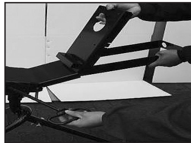
Step 8 Connect Gear Motor Mounting Base to Swivel Bracket Using the Pivot Pin.
