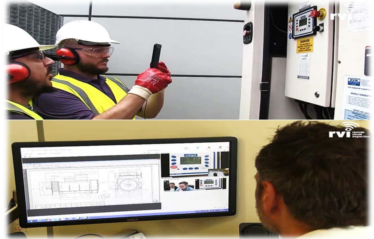
Figure.7 Remote Visual Inspection (RVI) deploys Fluor's Virtual SME tool, camera-enabled smart devices and Wi-Fi connectivity to stream surveillance activities live.
