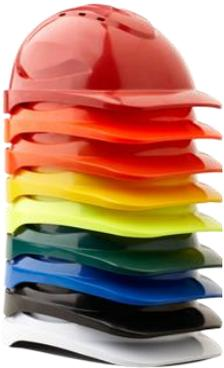
The Peak features a rain trough, HDPE shell, slots for accessories, 4 point suspension (3 levels for height adjustment), adjustment is a pin lock. ANSI Type 1 Class E certified.
