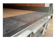
Our custom trailer threshold plates provides floor surface protection from forklifts . Its surface has a raised diamond design which creates a safe non-slip environment.
