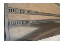
Engineered for truck or trailer fleets requiring extreme duty protection for sidewalls and flooring. Full-length (non-welded) scuff has no seams to snag and all holes are countersunk to protect fasteners.
