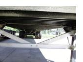
Light weight I-beams used as cross members in truck bodies and van trailers. These are the structural, load carrying components supporting the floor of the truck body or trailer. This material must be high strength, but light weight, in order to maximize the weight and volume of the cargo being hauled. Our cross members are in dry freight vans, flat bed trailers, truck bodies and cargo containers
