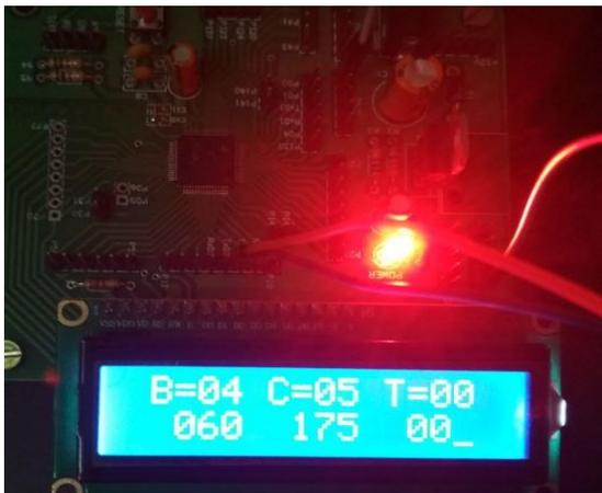
Fig 6: Vehicle count and toll charges on LCD. Vehicular and toll data uploaded to Amazon Web Sever
