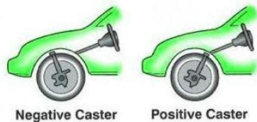
Figure 1.5: Wheel Alignment.
