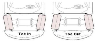
Figure 1.1: Toe Measurement.
