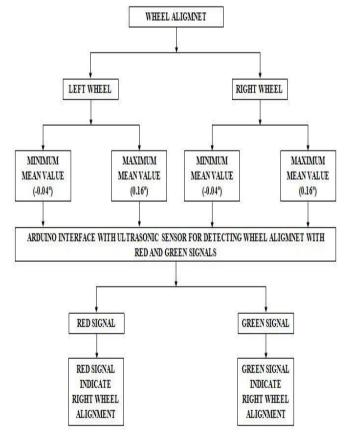
Figure 1.6: Flow Diagram of Work.
