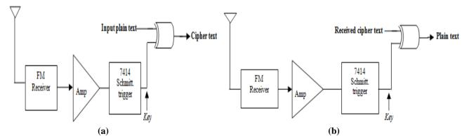
Fig. 4 Implementation of proposed circuit (a) Key used at authorised transmitter (b) Key used at authorised receiver
