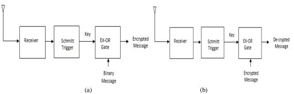
Fig. 3: Proposed technique (a) Key used at authorised transmitter (b) Key used at authorised receiver
