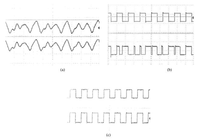
Fig. 5 Waveforms generated by two FM receivers operated separately. (*Upper: Demodulated at transmitter*) (*Lower: Demodulated at corresponding receiver*) (b) Encryption at the transmitter (*Upper: Plain Text signal*) (*Lower: Encrypted signal*) (c) De-cryption at the receiver (Upper: Plain text data transmitted at the sender) (Lower: De-crypted data at the receiver)
