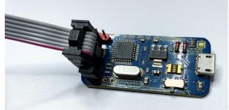
The picture below shows the 2x3 pin IDC cable from the USBASP programmer connected to the main board. The location of the RED stripe is important, I am using the red stripe to indicate VOUT / +5v from the USBASP programmer.
