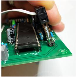
**NOTE!** The main board and IO/control board must be separated for programming to succeed. The IO board interferes with the pins required for programming.
