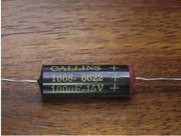
*Figure 6 1966 Callins miniature electrolytic capacitor*
