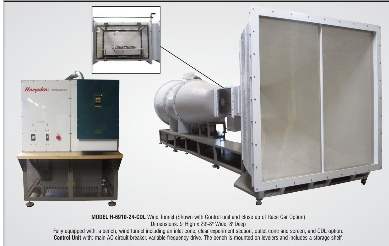
**MODEL H-6910-24-CDL** Wind Tunnel (Shown with Control unit and close up of Race Car Option)
