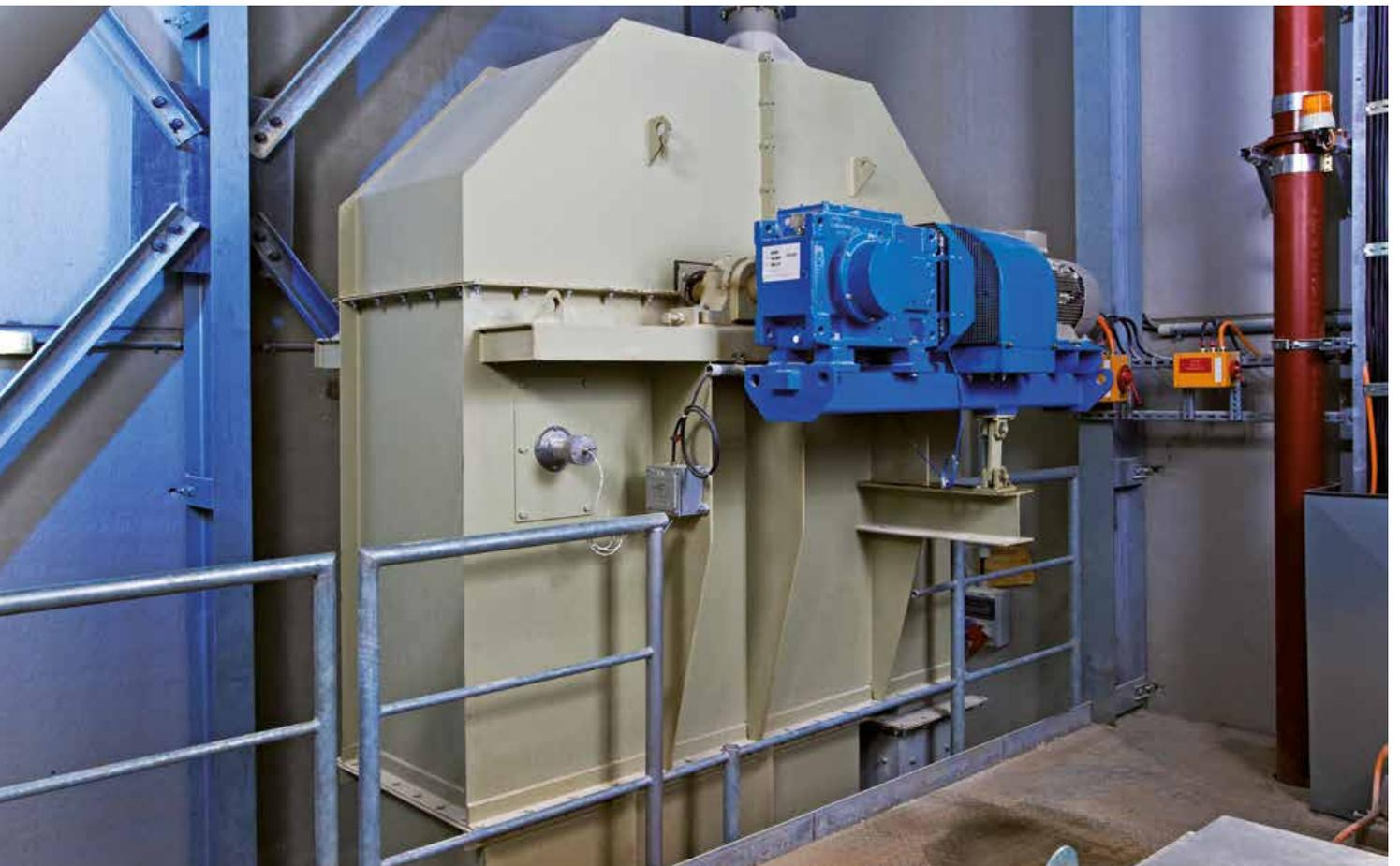
Bucket elevator head with single drive
