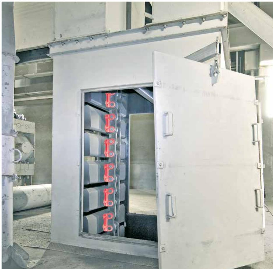
AUMUND Bucket Elevators with central chain are the ideal solution to raise granular, coarse and abrasive materials.
