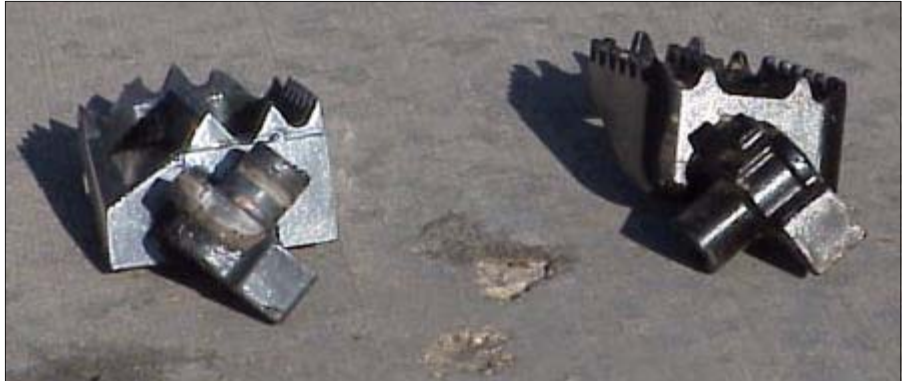
Modified IMS Peg left, Stock peg right
