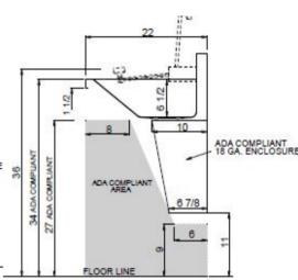
Engineering Specification: ADA COMPLIANT WALL HUNG SINK; 16 GA. 304 SS WITH 18 GA. 304 SS ENCLOSURE; FULLY WELDED & GRIND AND POLISHED TO A # 4 SATIN FINISH; 1-1/2" BULT IN GRID DRAIN.SENSOR FAUCET (AC OR BATTERY) WITH MIXING VALVE; EMERGENCY EYE WASH NOT INCLUDED.
