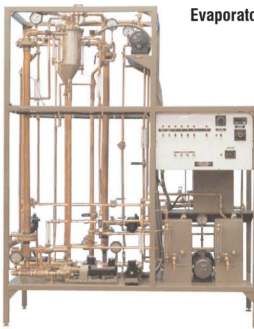
MODEL H-6140 Double Effect Evaporator Demonstrator shown without insulation Dimensions: 100"H x 72"W x 32"D - Shipping Weight: 1500 lbs.
