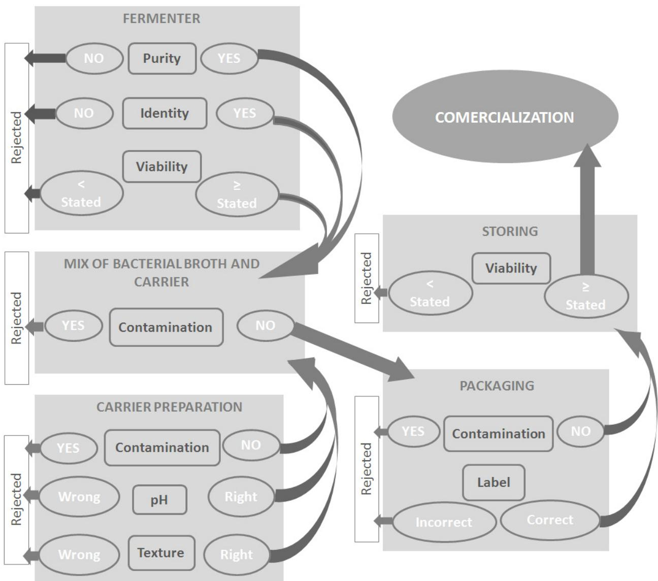
**Figure 2. Quality control in the biofertilizer manufacturing process.**
