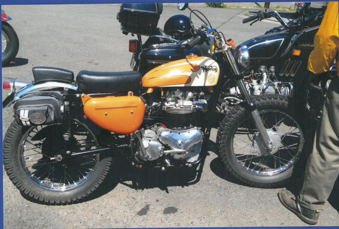
N15 Norton Oil tank, Bater front end, headlight from 1937 Dodge car, & instrument panel from Home Depot bucket!
