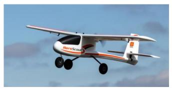
43" wingspan, SAFE technology, EPO foam construction, 3 cell electric
