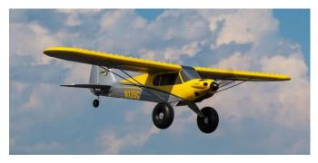
51" wingspan, SAFE technology, EPO foam construction, 3 cell electric, optional flaps
