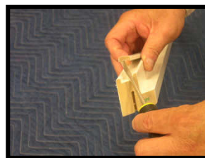
Lightly lift the screwdriver and pop off insert.
