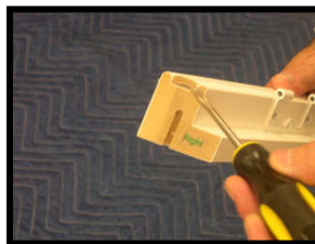
Use screwdriver to insert between insert and frame.
