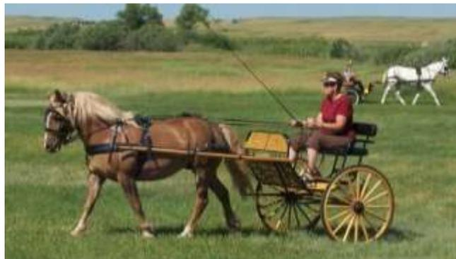
Shafts, 77" long -- Shaft width at cart end, 38" -- Shaft width at narrowest, 27" -- Width of cart floor, 40"
