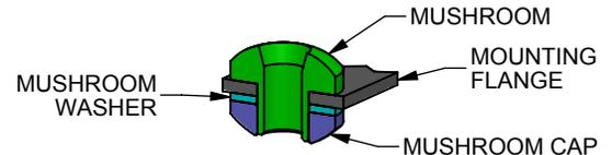
**FIG 2D: ALTERNATE INSTALLATION**
