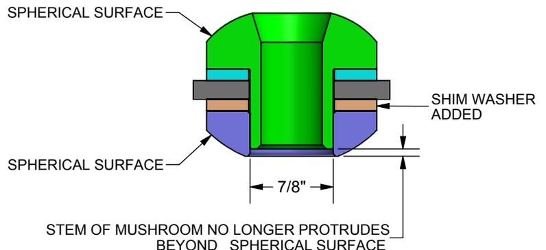
**FRONT SHOCK INSTALLATION (cont):** Next, insert the shaft of the shock absorber through the hole in the cup washer and slide it through the hole in the spherical surface (see FIGs 5 & 6). Place the other cup washer over the shaft of the shock that is sticking through the spherical surface and install a nut on the shaft.
