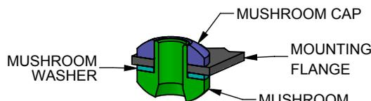
**FIG 2C: ALTERNATE INSTALLATION**
