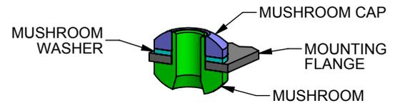
**FIG 2B: ALTERNATE INSTALLATION**
