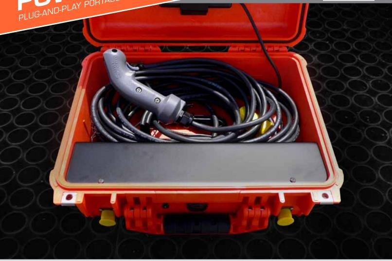
The Bambi Bucket® Power Pack is a portable and rechargeable power supply used in the operation of the Bambi and Bambi MAX buckets allowing them to be operated independently of the helicopter power supply. It consists of a battery pack, battery charger, bucket wiring harness and remote dump switch.
