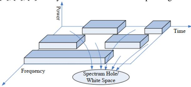
Fig.2 Spectrum Hole Concept
