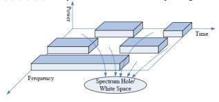
Fig.2 Spectrum Hole Concept
