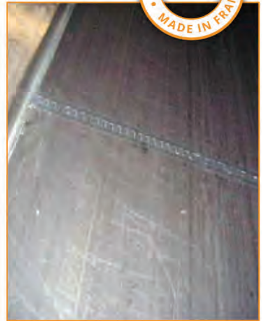
PVC splice in an airport belt
