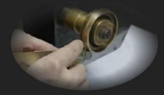
Comparing with diamond dull point, the jewelry processing efficiency of the diamond dull wheel is 5-10 times higher.
