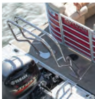
SKI TOW BAR This incredibly rugged and very stylish tow bar gets the rope above the motor and wake and will pull you anywhere you want to go.
