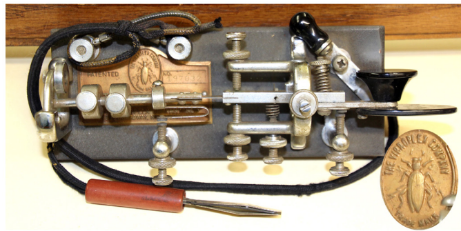
I. J. Carey's Vibroplex "BUG" Around 1908, telegraphers nicknamed these instruments "bugs" because they frequently sounded like one on a circuit. The Vibroplex Company adopted the bug as its trademark when it released its first keys for sale in 1905.
