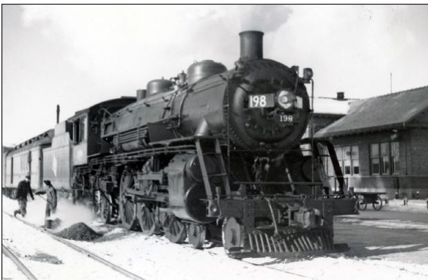
Passenger Train 4-6-2 locomotive #198 in front of the Mitchell, SD Depot March 1948 C.M.StP.&P.RR
