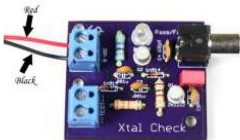
Photo # 1 Connecting power to the tester
