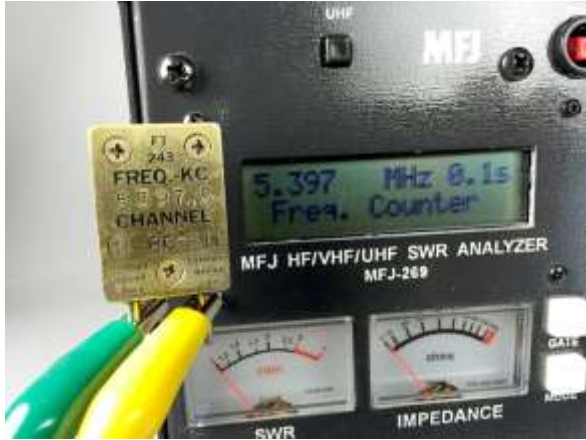
Photo # 3 Measuring Frequency of a FT 243 style crystal
