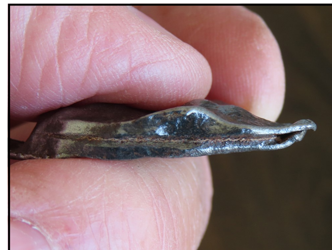
A seam between to the two pieces.
