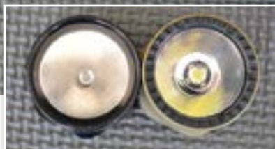
Incandescent (left) and LED (right).
