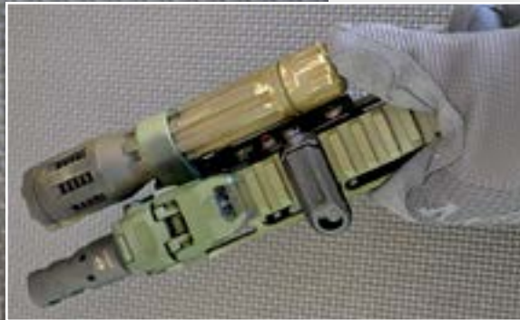
top: Mount the light far forward to minimize light masking.
