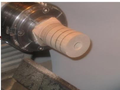
5) Now drill a 5/8" hole to within 1/8" of the base of the globe. This makes the globe easier to hollow since the center has been removed. It also sets the depth for hollowing.
