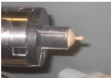
7) Finally screw the screw eye into the finial. I find this is easier while the finial is in the chuck because you can hold the screw eye still and turn the finial using the handwheel on the lathe.
