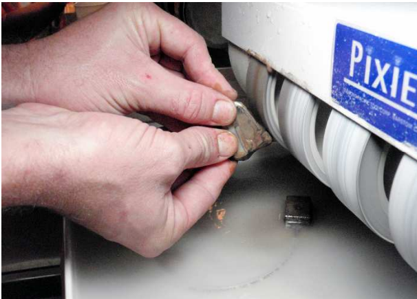
Grinding a rock to shape on the Pixie machine
